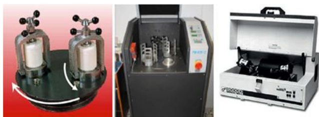
Figure 3: contains pictures of planetary and shaker mills.
