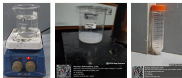
Figure 1: Preparation of chemically synthesized TiO 2 Nanoparticles (NP).
