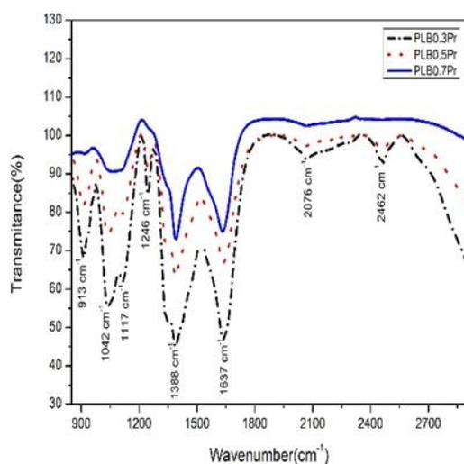
**Figure 2:** Fourier transform infrared spectrum of the Pr<sup>3+</sup> doped PLB glass system
