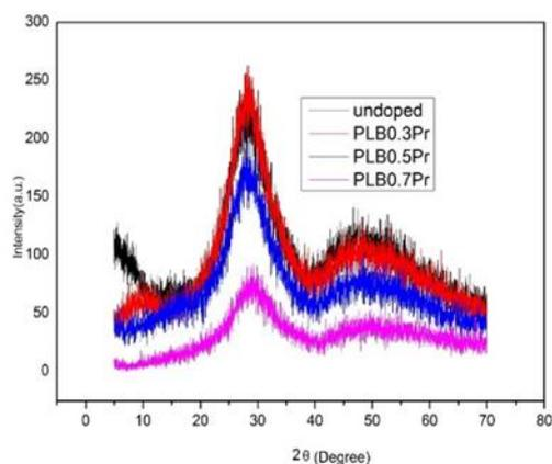
**Figure 1:** XRD patterns of Pr<sup>3+</sup> doped PLB glass system
