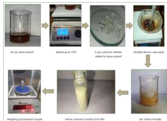
Figure 3: The process of making ZnO NPs from Ocimum Tenuiflorum leave extract
