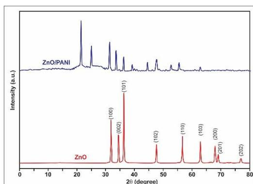
**Figure 1:** XRD spectra of ZnO and ZnO/PANI nanocomposite.
