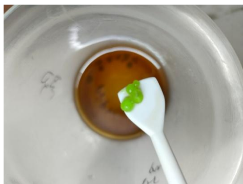
Figure 1: MOFs prepared using solvothermal method
