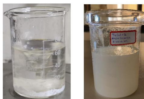
Figure 2: Transformation of Sol to Gel.
